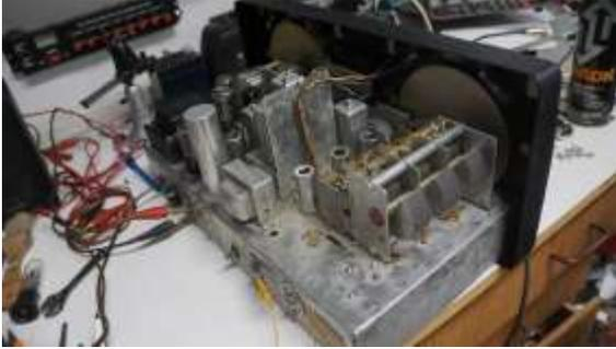
I removed the chassis from the cabinet, and separated the front panel. Then I sanded and wire brushed the panel and cabinet, and repainted it with a pretty close match to the original paint.
